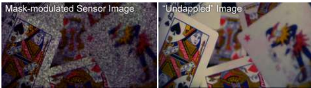
Figure 13: “Undappling” a mask-modulated sensor image (left). The known projection of the mask pattern can be divided out; remaining noise patterns in out-of-focus regions are further reduced using a coupled dictionary method (right).
