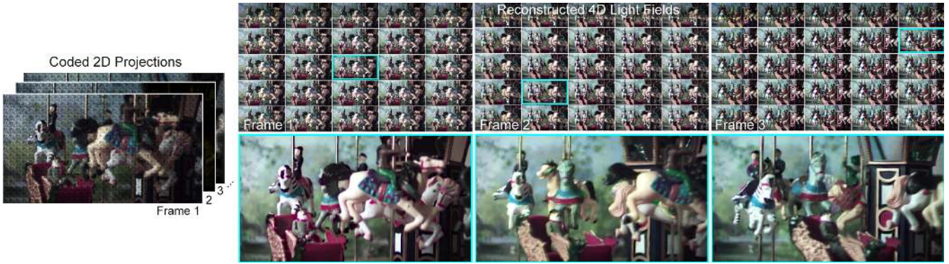
Figure 12: Light field reconstructions of an animated scene. We capture a coded sensor image for multiple frames of a rotating carousel (left) and reconstruct 4D light fields for each of them. The techniques explored in this paper allow for higher-resolution light field acquisition than previous single-shot approaches.
