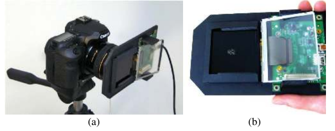
Fig. 2. (a) Our prototype camera where an LCD array is mounted to the lens of a digital camera. (b) LCD array showing an example mask combination.
