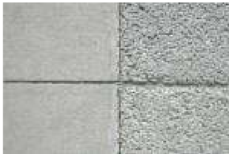
Figure 1.1.2 Comparison of Conventional Concrete and Pervious Concrete
