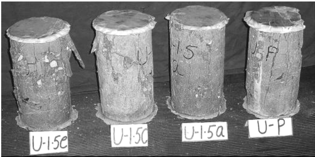
Fig. 18 Typical failure modes.
