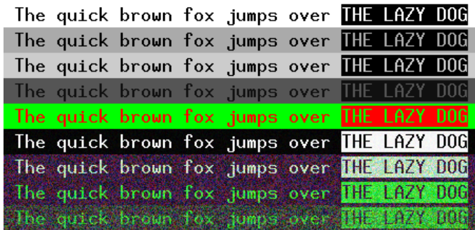
Figure 4.9: Example test image for text contrast in compromising emanations from DVI cables.
