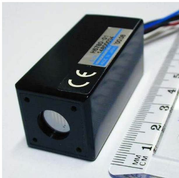
Figure 6.1: The Hamamatsu H6780-01 photosensor module used for these experiments contains a photomultiplier tube together with a high-voltage power supply.
