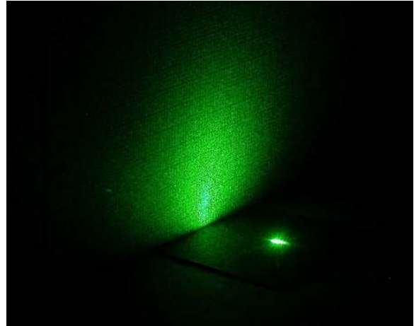
Figure 4: Reflection pattern on a real plain orange cardboard sample for an incident angle of about 20 degrees. Note that as no fluorescent surface is involved, both the immediate bright dot on the material and the reflection pattern are monochromatic green with no hints of orange. This photograph is to be compared with the one of figure 5 which involves a fluorescent day-glo orange cardboard sample.
