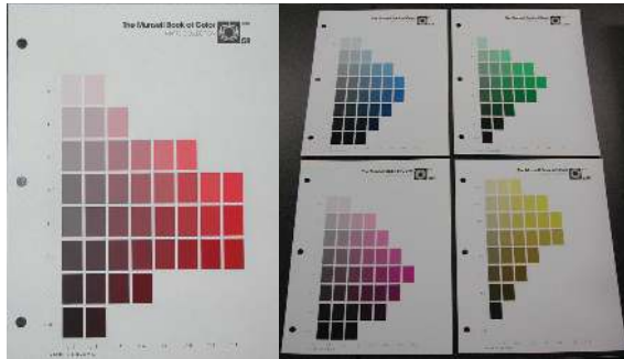
Figure 3: An example of a traditional COS: some pages from the matte Munsell Book of Color.
