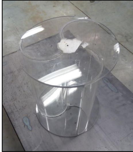
FIGURE 3-14: Fabricated Model of Semi Circular Bladed Rotor
