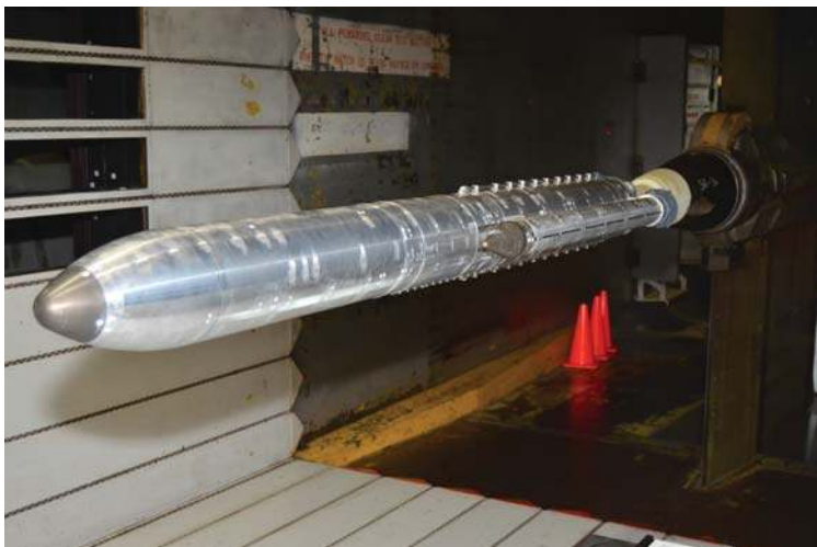
Figure 4: Photograph of SLS configuration installed in the Ames 11-Foot test section.
