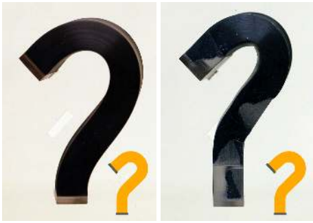
Figure 6: 3D printed example of a straight bar with uniform (left) and optimized (right) material distribution that is bent into a question mark shape by applying force only on its end caps. The small orange icon shows the target shape.
