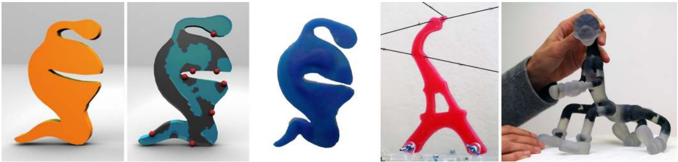
Figure 1: We present a method to convert animated digital characters into physically fabricated prototypes. Our physical characters can be actuated using pins, strings, or posed by hand.
