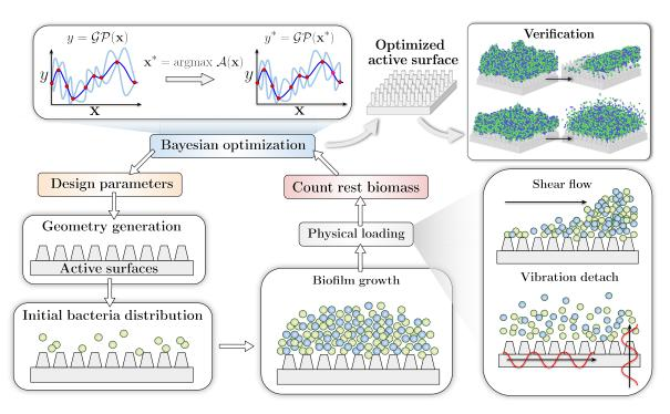
Figure 3: The schematic for the BO workflow for designing antimicrobial surfaces based on LAMMPS and Python. The optimization begins with randomly initiated geometries represented via the design parameters. The bacteria cells are initiated on top of the nanosurface and grown and removed via different physical loading. The remaining bacteria cells are the objective for the optimization. The optimized geometries are then verified through numerical simulations.
