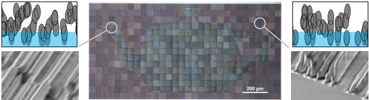
Fig. 1. (Center) Microscope image of a structurally colored surface with the corresponding nanostructures of the fore- and background depicted left and right of it. (Top) The cross-sectional profiles of both transparent structures were designed with our method using full electromagnetic simulation. (Bottom) Micrographs of the fabricated nanostructures with a length scale of 5 µm across the image diagonal.
