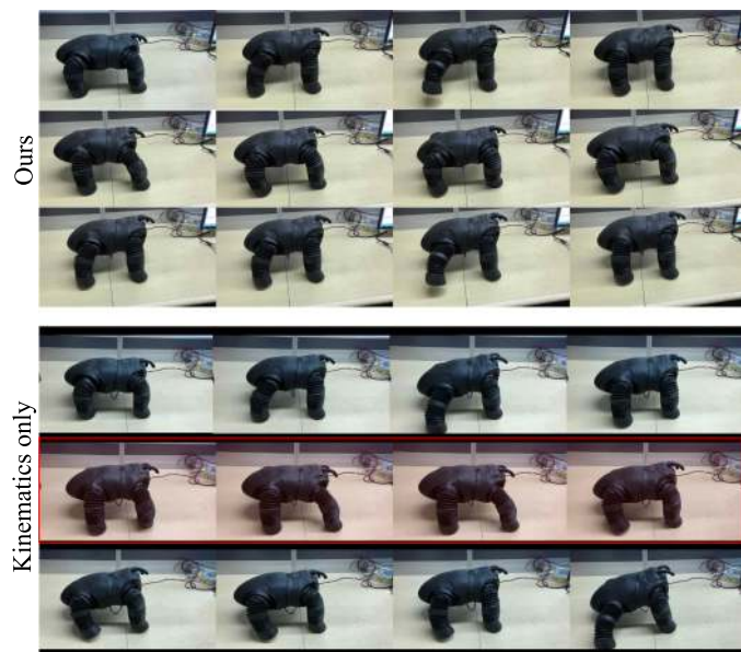
Fig. 19. Physical experiments show that kinematic-only optimization is not a feasible solution for skinned robots – there are noticeable back steps (highlighted with a red box) in a motion cycle as the driving torques, after damped by the skin deformation, are not strong enough to produce necessary normal contact forces. Please refer to the accompanied video for a clearer comparison.
