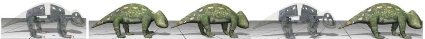
Fig. 14. The motion of a lizard-like robot. We edit the second template in Fig. 6 with SolidWorks scripts to create the design of its mechanical skeleton. With user provided inputs, our system generates plausible motions of this robot.
