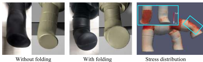
Fig. 17. Adding folding regions significantly relieves the stretching stress over the skin. We program the motor at an ankle joint of the beetle-like robot to rotate \pm 70^\circ within 2 seconds in this experiment. A smooth skin can only be bent around \pm 20^\circ , while the folded skin is able to reach the desired deformation. The physical experiment (black skins) results are consistent with simulation results (yellow skins).
