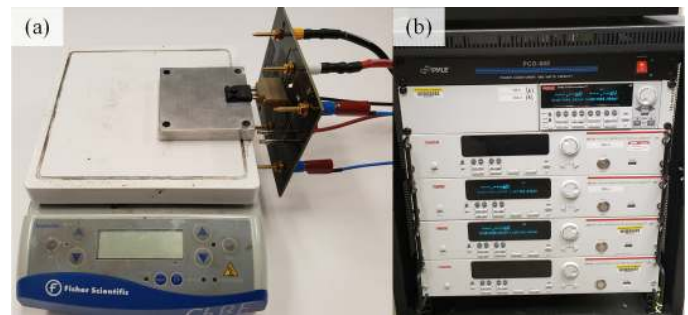
Fig. 1. Experimental test setup, (a) C2M0025120D mounted to hotplate, (b) Keithley Semiconductor Characterization System (SCS)
