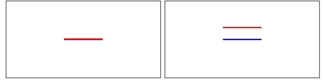
Fig. 10 Hypothetical case of two bars that are initially coinciding, with one hole in the fluid mechanics domain (left). Then the red bar starts moving upward, creating a second hole in the domain (right)
