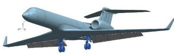
c) 39° deflected flaps with main gear deployed. Left image, 2006 flight test and right image, simulated model.
