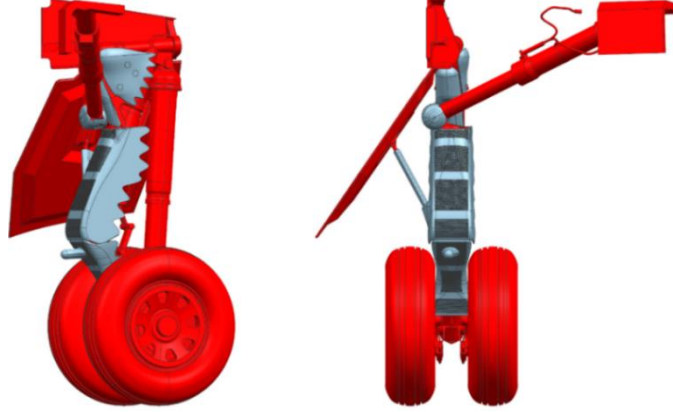
Figure 3. Full-scale versions of upper and porous knee fairings.
