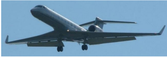
c) 39° deflected flaps with main gear deployed. Left image, 2006 flight test and right image, simulated model.
