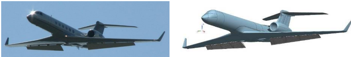
a) 39° deflected flaps with main gear retracted. Left image, 2006 flight test and right image, simulated model.
