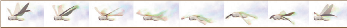
Figure 2: Flight of an insect: vorticity at eight instants during the flapping cycle. This figure appears as Fig. 7.26, p. 189, in the book
