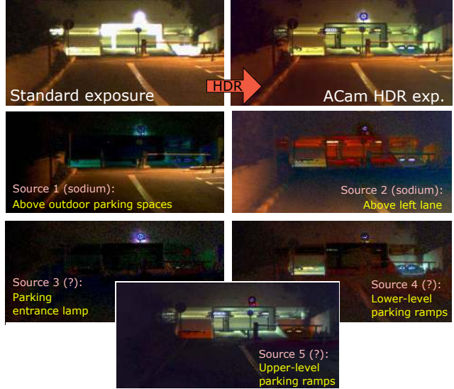
Figure 10. An unmixing experiment for a scene that deviates from our assumptions. Here, some scene bulbs are not in DELIGHT and are not observed directly due to their location deep inside the building. Lacking knowledge of the number of independent sources, BRFs and chromaticities, we set S = 5 for unmixing but in reality S is likely higher. The results suffer from residual crosstalk and color distortion, e.g., notice that some signal from sources 4 and 5 falsely appears in parts of sources 1 and 2.
