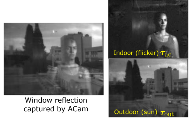
Figure 6. Temporal variations due to AC flicker are attributed to the indoor scene. ICA separates the indoor reflection from the transmitted scene. Both are recovered up to an unknown scale.
