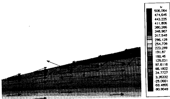
(d) Reverse flow on divergent wall, u-velocity vectors. Figure 5. NPR=3.6, M=0.3 , no injection.
