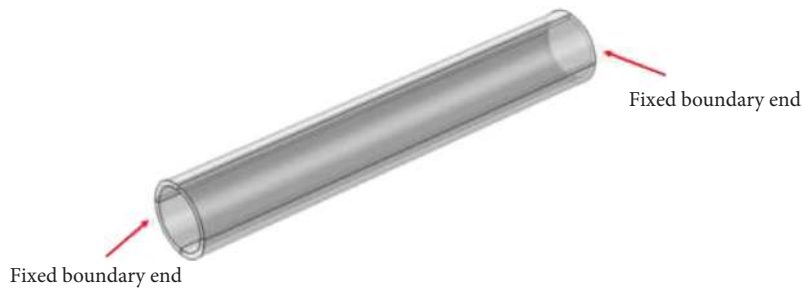
FIGURE 8: Fixed-fixed boundary fundamental frequency analysis (both the ends are fixed).
