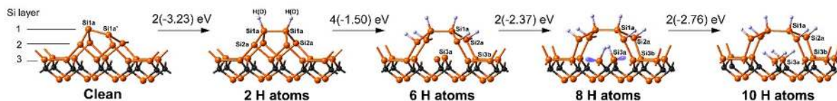
Fig. 11. Formation of nanotunnel on SiC(001) 3 \times 2 surface by successive hydrogenation. Color code: orange: Si, black: C, white: H, blue: dangling bonds.
