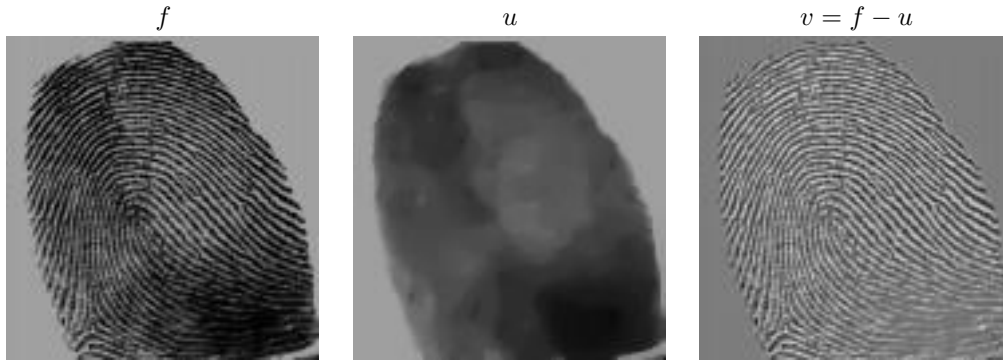
Figure 7. Exact image decomposition into cartoon and texture using the (BV, BV^*) minimization model. Left: real fingerprint data. Middle: cartoon component u . Right: oscillatory component v = f - u (+125).
