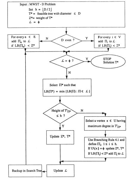
Figure 4.2: Flowchart of Branch and Bound Algorithm.
