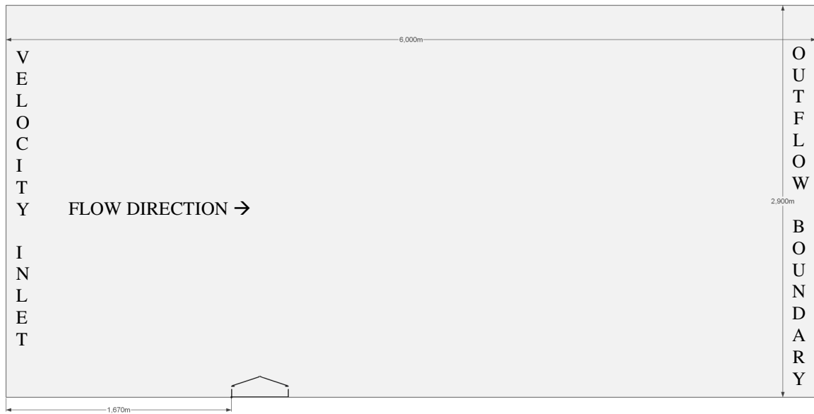
Fig. 2. Computational domain, i.e. the second half of a wind tunnel's test section (6 m x 2.9 m), with a scale model positioned at 1.67 m from the velocity inlet boundary.
