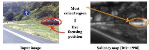
Fig. 1 One promising way of understanding human visual attention based on visual saliency. The model assumes that for a given input image (left) a gray-scale image called a saliency map (right) is automatically calculated in the brain, and we would first pay attention to the position yielding the maximum pixel value in the saliency map.
