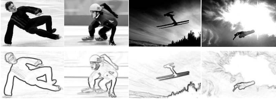
Figure 1.1: Images of simple foreground and background can be segmented based on feature attributes, such as brightness and spatial coherence. Row #1: images. Row #2: edge magnitudes obtained at a fixed scale. Same convention for Fig 1.2 to Fig 1.4.
