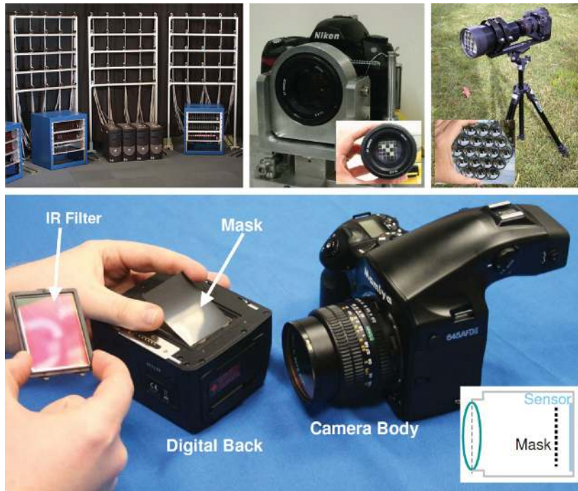
Figure 4: Light field cameras can be categorized by how a 4D light field is encoded in a set of 2D images. Methods include using multiple sensors or a single sensor with temporal, spatial or frequency-domain multiplexing. (Top, Left) Wilburn et al. [WSLH02] describe a camera array. (Top, Middle) Liang et al. [LLW*08] achieve temporal multiplexing with a programmable aperture. (Top, Right) Georgiev et al. [GIBL08] capture spatially multiplexed light fields using an array of lenses and prisms. (Bottom) Raskar et al. [RAWV08] capture frequency-multiplexed light fields by placing a heterodyne mask [VRA*07, VRA*08, LRAT08] close to the sensor. (Figures reproduced from [WSLH02], [LLW*08], [GIBL08] and [RAWV08].)
