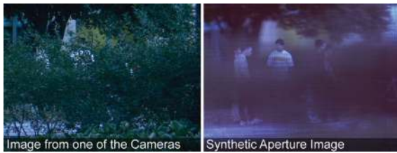
Figure 6: The images of a light field can be processed to reveal parts of the scene (right) that are occluded in any of the individual views (left) of a camera array. (Figures reproduced from [VWJL04].)
