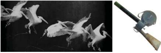
Figure 8: Multiple frames of a flying bird multiplexed into a single photograph (left). These kinds of photographs were shot with a photographic gun (right) by Etienne-Jules Marey as early as 1882.
