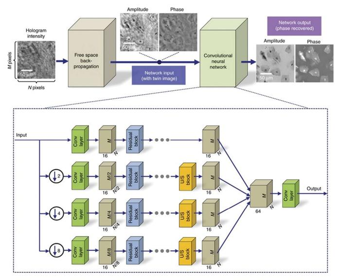
Figure 3. CNN architecture to recover complex-value information of the object [59].
