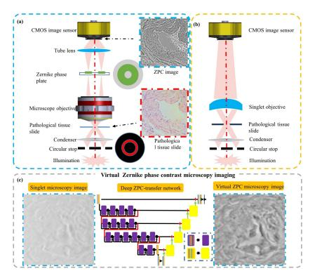
**Figure 18.** Singlet virtual phase-contrast microscopy. [108]: (**a**) a 2D schematic of a traditional Zernike phase contrast microscopy setup, (**b**) a 2D schematic of a singlet phase contrast microscopy setup, and (**c**) Deep ZPC-transfer network architecture.
