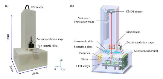
Figure 16. Singlet multi-spectral microscopy [107]: (a) photograph, and (b) a 3D mechanical design.
