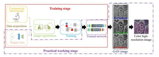
**Figure 13.** Deep learning architecture to enhance high-resolution and image contrast for the singlet bright-field microscopy in Figure 12 [105].
