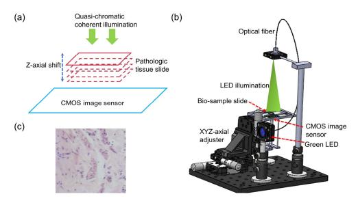
**Figure 2.** Typical schematic of lens-less diffraction microscopy setups based on multiple holograms: (a) the principal schematic; (b) a 3D mechanical design of a lens-less diffraction microscope; (c) typical H&E stained pathological slide [57].
