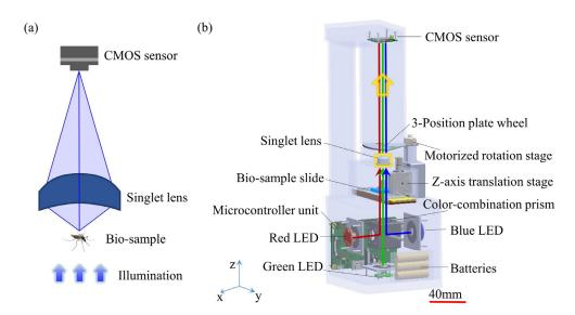
**Figure 12.** Singlet bright-field microscopy setup [105]: (**a**) a 2D principle schematic and (**b**) a 3D mechanical design.
