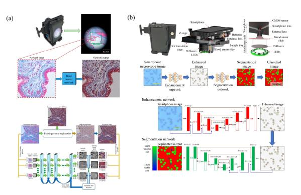
**Figure 8.** Smartphone-based bright-field microscope with deep learning. (a) Deep learning enhanced mobile-phone microscopy [77], and (b) a photograph of the smartphone-based bright-field microscope. [78].
