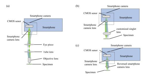
**Figure 7.** Smartphone platforms based on: (**a**) commercial microscopic objective lenses, (**b**) customized single lenses, (**c**) inverted pinhole lenses.
