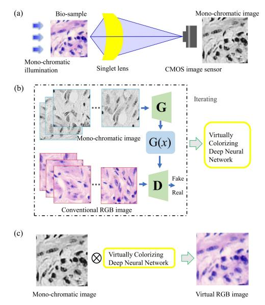
**Figure 14.** Singlet achromatic microscopy based on deep learning virtual colorization [106]. (**a**) 2D schematic; (**b**) a deep learning virtualizing flowchart; and (**c**) an application working flowchart.
