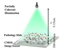
Figure 1. Typical schematic of lens-less diffraction microscopy setups based on a single frame [39].
