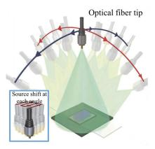
Figure 20. Super-resolution lens-less microscopy based on multi-angle scanning [122].
