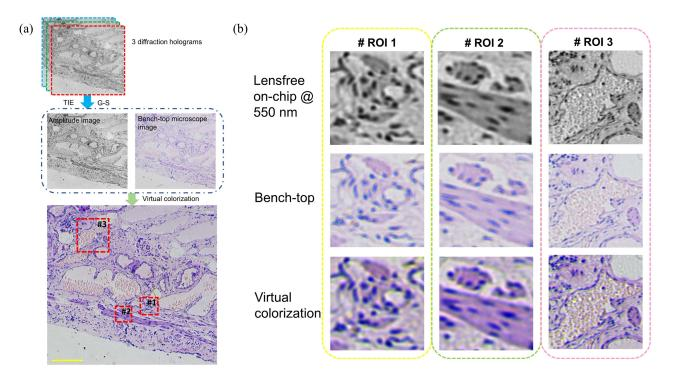
Figure 4. (a,b) Deep learning virtually colorizing to achieve colorful lens-less microscopy [57].
