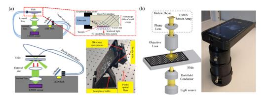
Figure 10. Smartphone-based dark-field microscopy based on (a) external angular illumination [84], and (b) a dark-field condenser [83].
