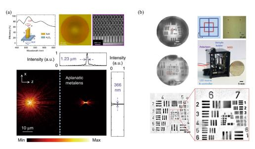
**Figure 19.** Portable singlet meta-lens microscopy setup: (**a**) macro-scale and nano-scale structure of a singlet meta-lens [110] and (**b**) a photograph of the singlet meta-lens microscopy setup with the resolution test result [111].
