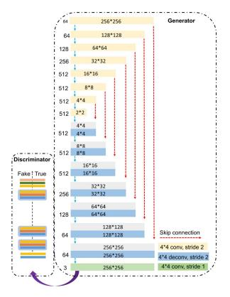
Figure 5. Deep learning virtually colorizing based on a GAN architecture [57].
