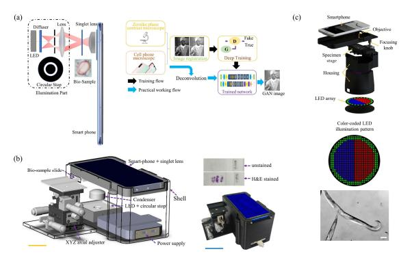
**Figure 9.** Smartphone-based phase contrast microscopy setups: (**a**) a 2D principle schematic based on a singlet objective and deep learning architecture for image enhancing [81]; (**b**) a 3D mechanical design [81]; (**c**) smartphone-based phase contrast microscope based on computational LED illumination [79].
