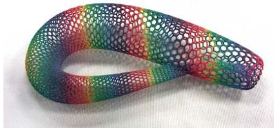
Fig. 9. 3D object printed using HANS3D pipeline to control voxel-by-voxel volumetric material composition (Model: Klein Bottle by krasul, published on July 22, 2013, www.thingiverse.com/thing:121871 under Creative Commons – Attribution license).
