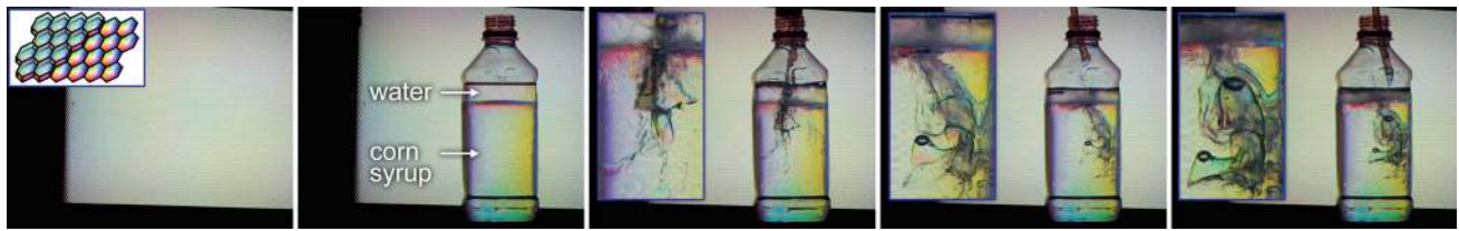
Fig. 10 The classic Rainbow Schlieren filter encoded in our light field probe can visualize magnitudes and angles of refractions in complex media such as this mix of clear corn syrup and water
