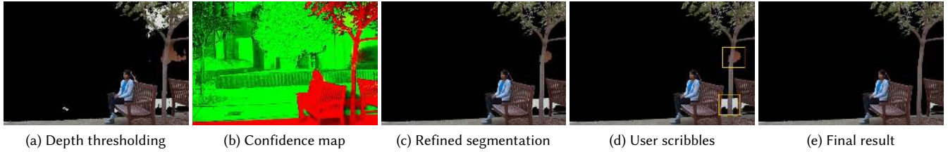
Fig. 9. Robust depth-based image segmentation. Accurate foreground/background segmentation with respect to a dolly plane is needed for synthesizing multi-perspective images. (a) A naïve segmentation by simply thresholding the depth-maps is brittle and results in artifacts. (b) A confidence map is obtained by warping the naïve segmentations from the other cameras and filtering them based on color similarity. Here, the intensity of red indicates the number of foreground votes, and green denotes background votes. A simple majority voting scheme gives us good segmentations, which is further refined with image matting, shown in (c). Nevertheless, if the depth for some regions is consistently wrong in multiple images, we will get wrong segmentation results. When this happens, we allow user to perform interactive segmentation by detecting the problematic regions as shown by yellow boxes in (d) and then providing foreground/background scribbles to get the final result shown in (e).
