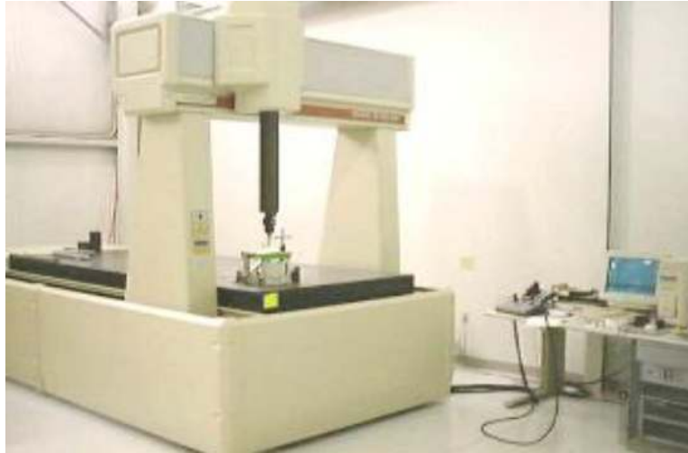
Figure 2.3: The Cordax RS-220 DCC Coordinate Measuring Machine (CMM).
