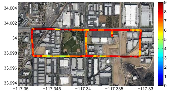
Fig. 5. Route and the satellite availability of the 640-s moving data experiment. The x - and y -axis are the longitude and latitude in degrees, respectively. The colors along the route indicate the number of satellites visible to the receiver at that location and time.
