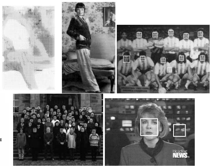
Figure 7: Top left: The intensity values of the pixels of the left image are proportional to the number of reduced set vectors used to classify their associated patches of the middle image. Light grey corresponds to the use of a single reduced set vector, black to the use of all the vectors. Top middle: 153 \times 263 middle image contains 76108 patches and was detected in 2.58s. Top right: A 601 \times 444 image containing 518801 patches detected in 27.9s. Bottom Left: 1280 \times 1024 contains 2562592 patches and was detected in 80.1s. Bottom right: A 320 \times 240 image containing 147289 patches detected in 10.4s (Note the false positives).
