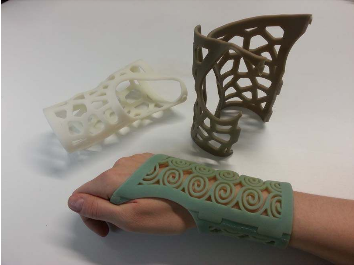
Figure 7: Proof-of-concept AM wrist splint prototypes
