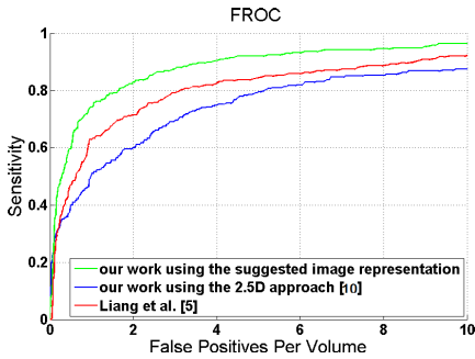
Fig. 4. Our CAD system using the suggested image representation outperforms the best hand-crafted approach [5] and also a CNN powered by a 2.5D approach [10].
