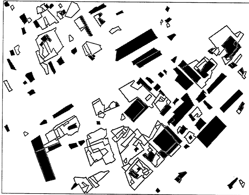
Figure 31: Detected segment cycles in the image of Figure 16; building-like cycles are filled in black.
