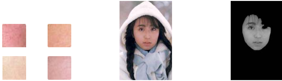
Figure 2. Skin regions found (right) in an input image (centre) using a statistical model built using sample skin images (some of them on the left).
