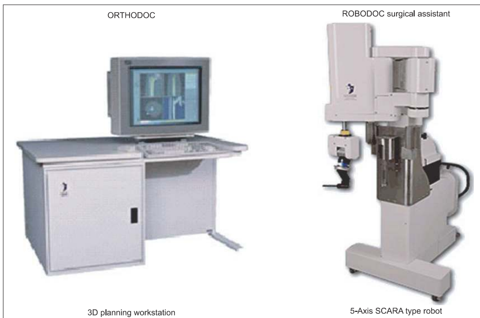
Fig. 1. The ROBODOC system including ORTHODOC, a 3-dimensional (3D) preoperative planning workstation, and ROBODOC surgical assistant, a 5-axis SACARA type surgical robot.
