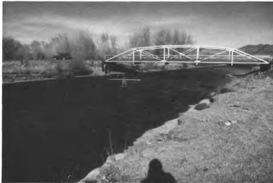
Figure 3.--Downstream view on White River above Coal Creek near Meeker, Colorado. Photograph taken during low flow with rod held at level of n-verification measurement.
