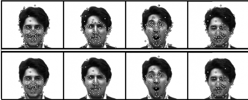
Fig. 4. SIFT descriptors of a person of the YALE database. The top row shows all descriptors found while the bottom row shows only the descriptors selected by the proposed method
