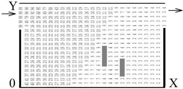
Fig. 3. Substrate concentration in the bioreactor (two plates, scenario no. 3)
