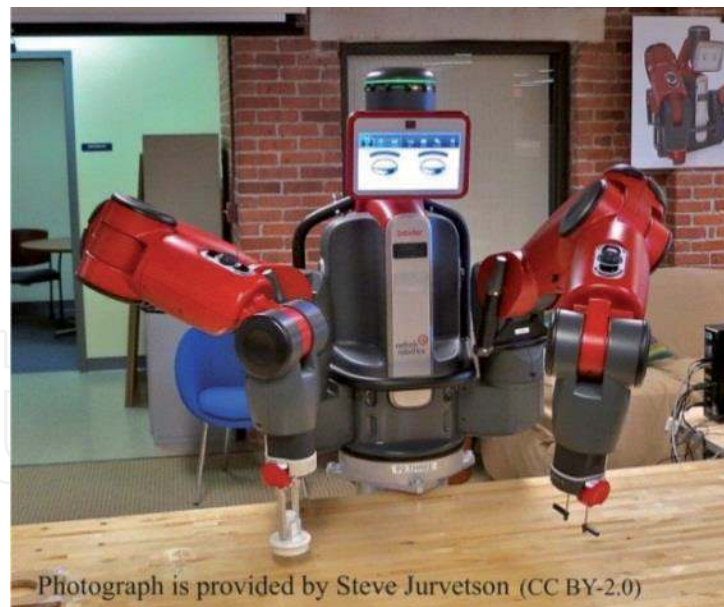
Figure 7. A collaborative robot: Baxter robot [52].
