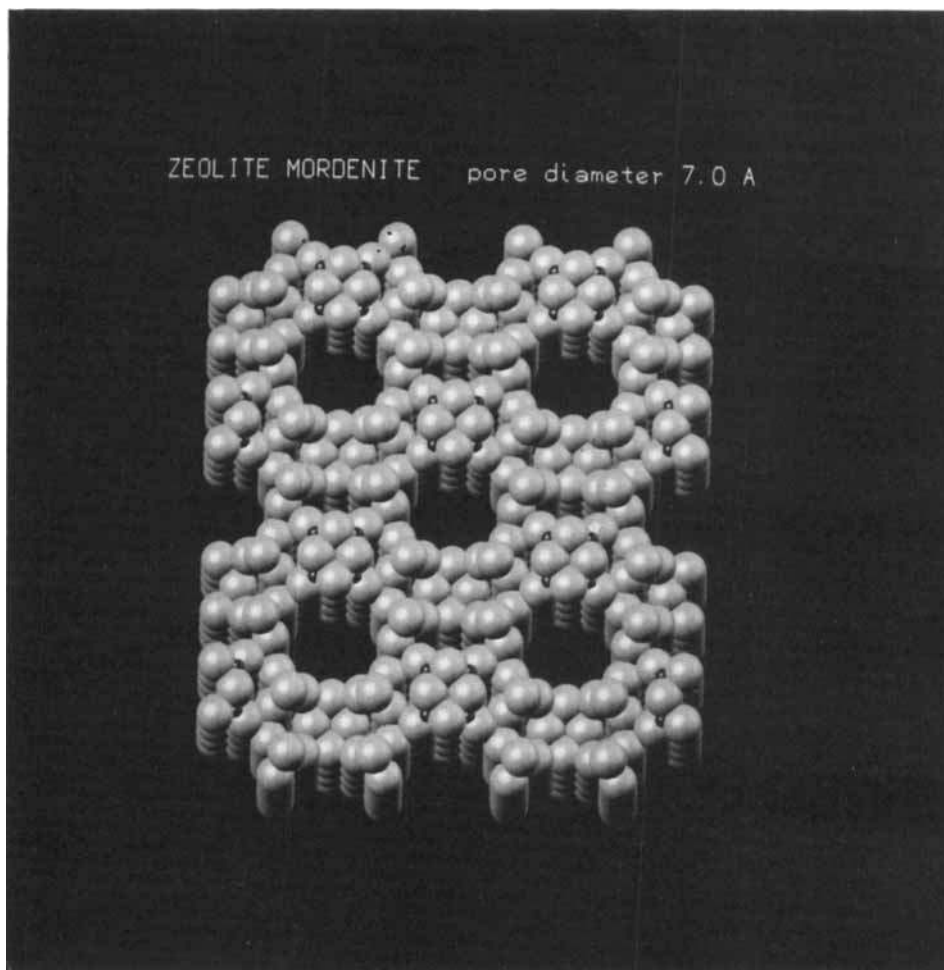
Figure 2 Structure of zeolite mordenite. The channel system consists of two types of channels which are parallel to each other (both viewed), the main channel has a pore diameter of 7 Å, whereas the secondary channel is much smaller. Side pockets are located at the edges of the main channels and are small cages with an entrance diameter of approximately 5 Å. Oxygen atoms are coloured yellow, T-sites (silicon or aluminium atoms) are tetrahedrally surrounded by oxygen atoms and are coloured red. (See colour plate VI.)
