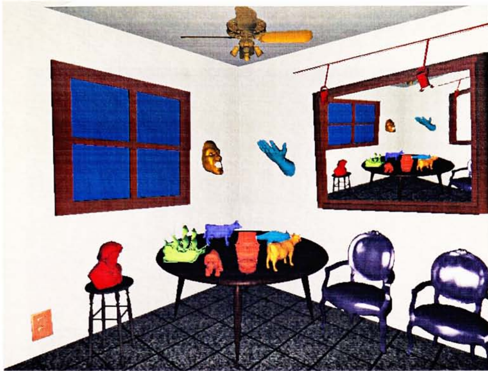
Figure 39. A more complicated scene, including metameretic, fluorescent, metallic, and texture mapped objects. The image on the wall is an actual full spectral texture map created using a multi-pass rendering technique. This scene is illuminated by CIE Illuminant D65.
