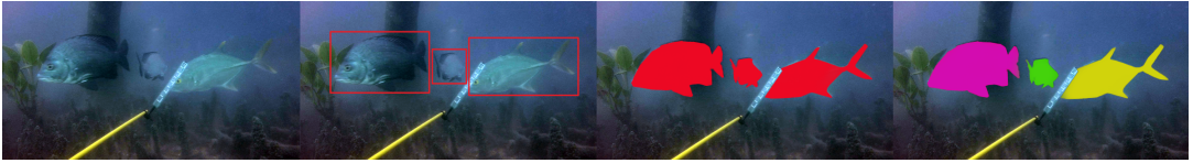
FIGURE 1 Illustration of four typical types of CV tasks From left: Image Classification ( i.e. is there a fish in the image, or what type (class) of fish is in the image?), Object Detection/Localisation, Semantic Segmentation, Instance Segmentation.
