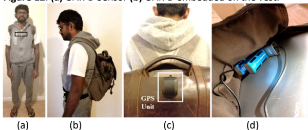
Figure 13: Physical setup showing (a) front view – sensors marked with black rectangular box (b) side view (c) GPS unit placed over the backpack and connected to the computing unit inside. (d) The computing unit inside the backpack along with NCS2s.
