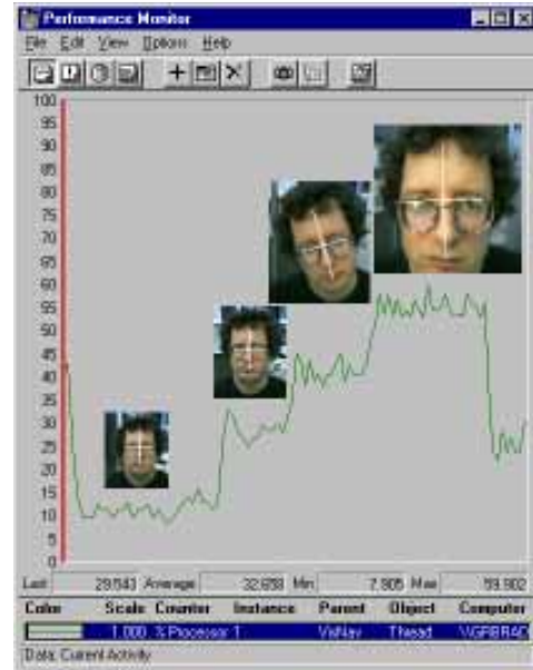
Figure 19: Performance scales inversely with tracked object size (ordinate is percent of CPU used)
