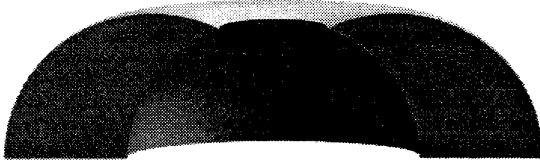
Figure 9: Candidate volume for one linear feature, considering only field-of-view and resolution constraints. The figure has been cut away twice to show the inside, but the actual volume is symmetric about the two cutaway planes.
