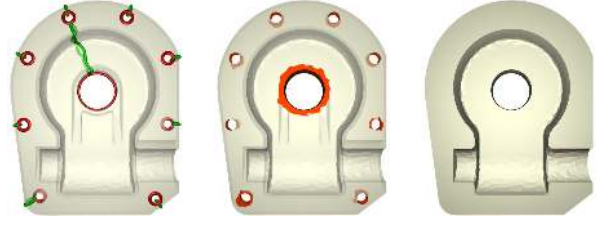
Figure 7: From left to right: handle and tunnel loops computed on Casting, tunnel features are identified, small tunnel features are filled.
