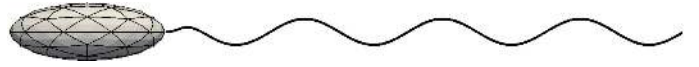
FIG. 4. Computational model II: Side view of the boundary element mesh of an E. coli bacterium with the cell body modelled as a surface distribution of stokeslets on a prolate spheroid and the flagellar filament modelled as a line distribution of stokeslet on the centreline of a rigid left-handed helix.
