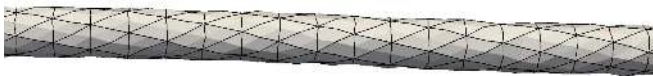
FIG. 8. Surface discretisation of a rigid helical object using 6-nodes curved elements. Evenly spaced circles are created along the centreline of the helix that are discretised into 12 points that either form a vertex or midpoints of the individual elements.
